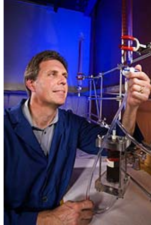
Agricultural engineer Barry Allred conducts an experiment to measure permeability (water flow capacity) of a filter material. (D1323-1)
