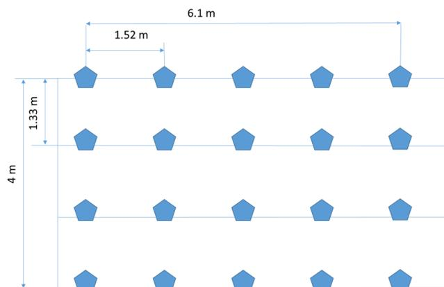
Figure 4. The layout of nozzles in rainfall simulator.
