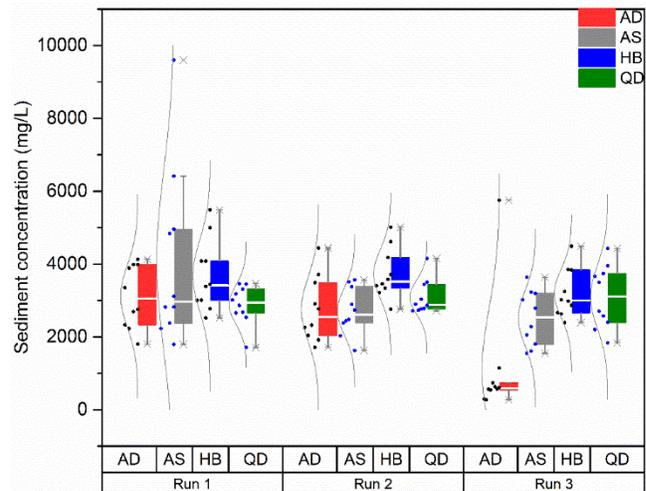
Figure 7. Grouped box chart of sediment concentration during the first three runs. (dot near box is the sediment concentration data for each inlet; the curve line is the distribution of the data; QD-QuickDrain low profile inlet, AD-AgriDrain wick inlet, HB-Hickenbottom standard inlet, and AS-Ag-Solutions standard inlet).
