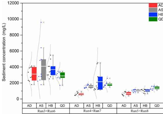
**Figure 9. Grouped box chart of sediment concentration data for combined runs. (dots near box is the sediment concentration data for each inlet; the curve line is the distribution of the data; QD-QuickDrain low profile inlet, AD-AgriDrain wick inlet, HB-Hickenbottom standard inlet, and AS-Ag-Solutions standard inlet).**
