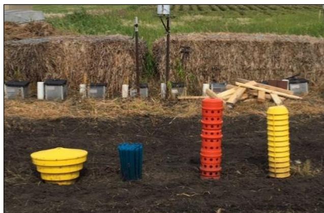
Figure 1. Surface inlets evaluated in this study. From left to right: (1) Ag-Solutions® QuickDrain® low profile inlet, (2) AgriDrain® wick inlet, (3) Hickenbottom® standard inlet, and (4) Ag-Solutions® standard inlet.
