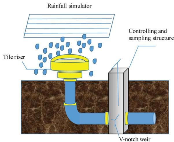
Figure 3. Schematic of field test site.
