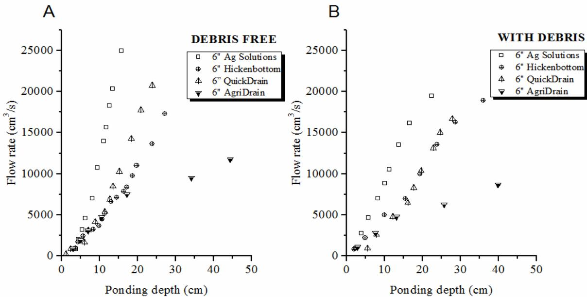
Figure 6. The ponding depth and flow rate relationship for different inlets during the debris free (A) and debris present (B) laboratory test.
