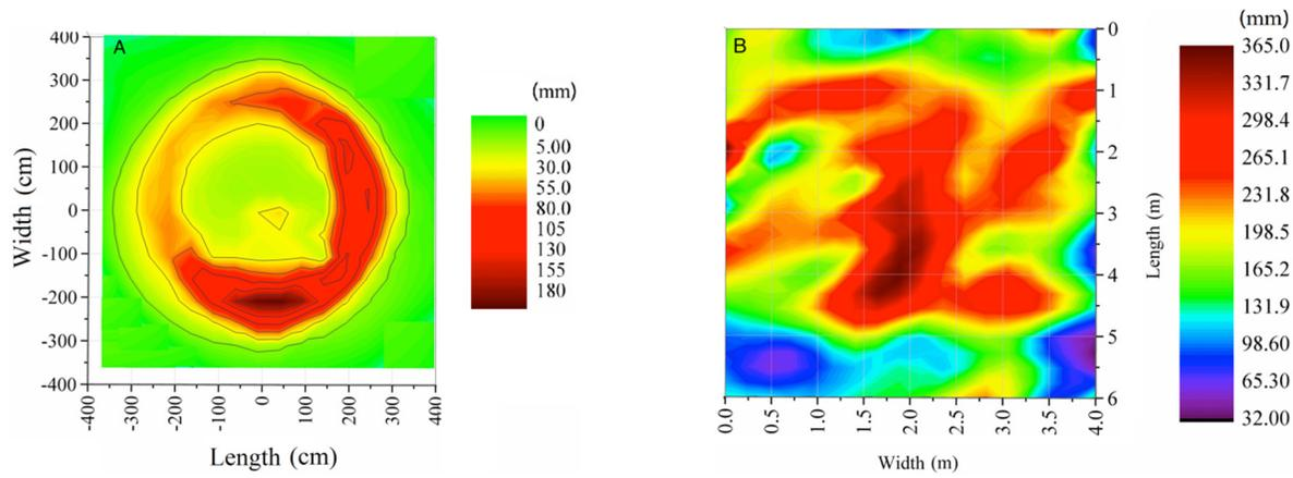
Figure 5. Rainfall distribution of a single nozzle (A) and simulation event (B).
