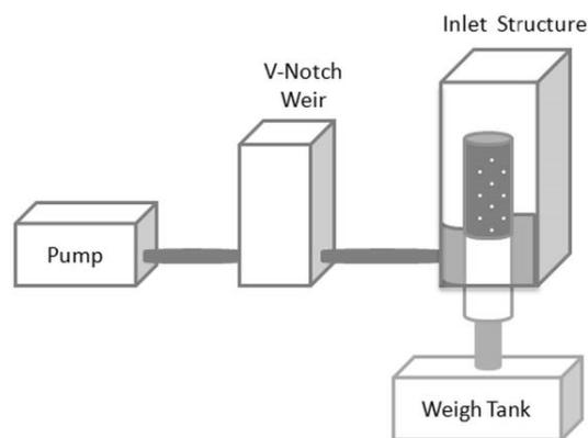
Figure 2. Schematic demonstrating set up for the laboratory test of inlets.
