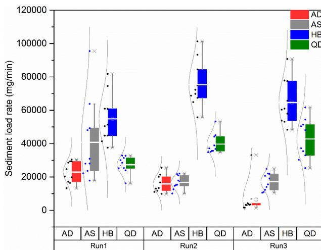
**Figure 8. Grouped box chart of sediment load during the first three runs. The white line in the middle of box represented the mean. (dot near box is the sediment concentration data for each inlet; the curve line is the distribution of the data; QD-QuickDrain low profile inlet, AD-AgriDrain wick inlet, HB-Hickenbottom standard inlet, and AS-Ag-Solutions standard inlet).**
