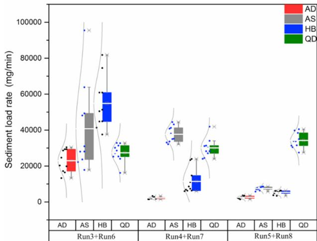
**Figure 10. Grouped box chart of sediment load data for combined runs (dot near box is the sediment concentration data for each inlet; the curve line is the distribution of the data; QD-QuickDrain low profile inlet, AD-AgriDrain wick inlet, HB-Hickenbottom standard inlet, and AS-Ag-Solutions standard inlet).**
