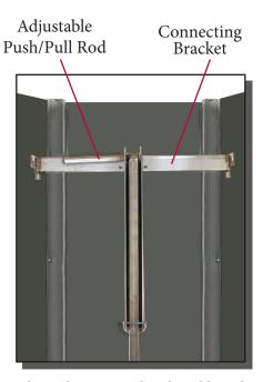
When valve is open, the adjustable push/pull rod locks in open or closed position.
