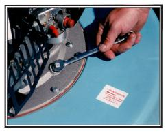
Your WATERMASTER Pump is shipped dry. Oil must be added to the pump's transmission and the engine crankcase.
