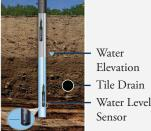
Fully automatic, completely buried, and can be used in series.
