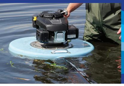
Powerful: Pumps approximately 840 gallons per minute through a 6"-diameter discharge hose.
